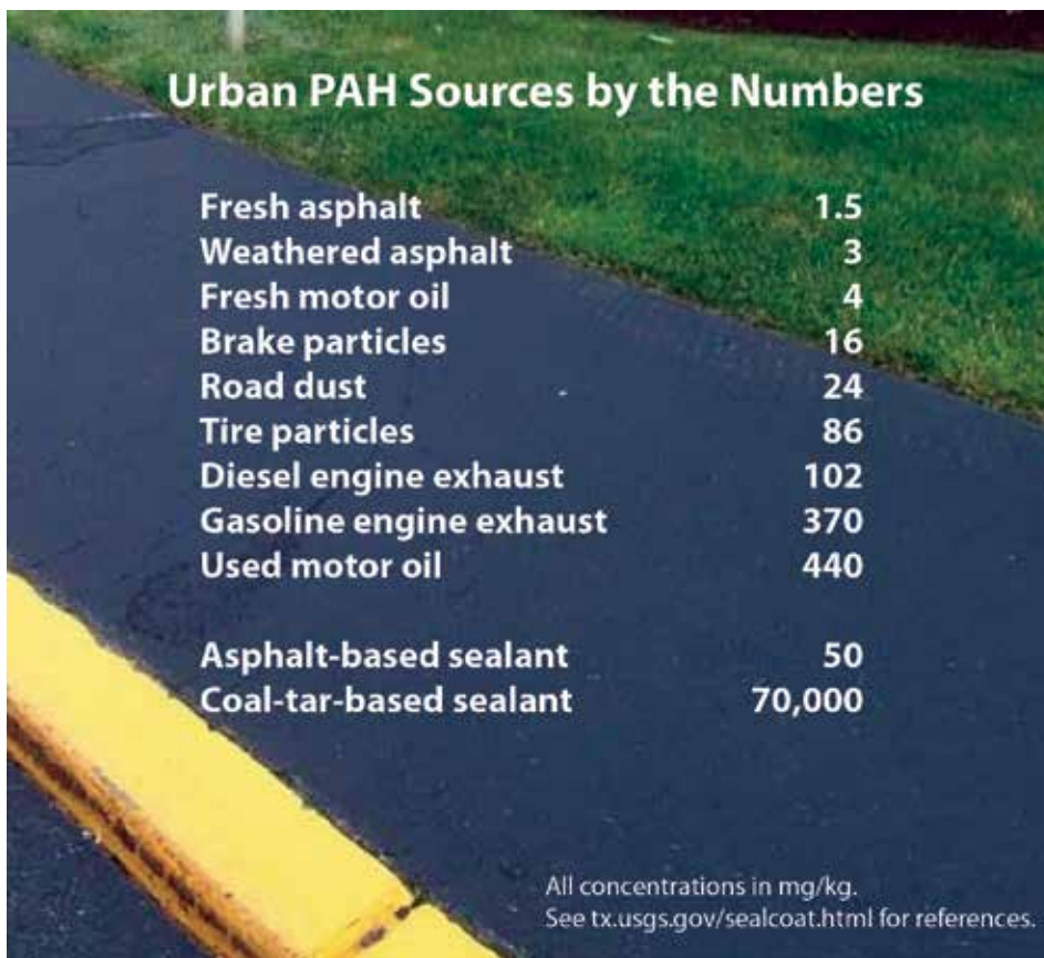
Figure 2. PAH concentrations in typical urban sources. The concentrations shown are a mean or median from as many as six studies.
