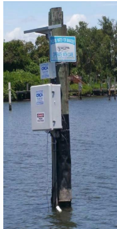
NuLab monitoring nutrients in a waterproof enclosure on a Florida bay
