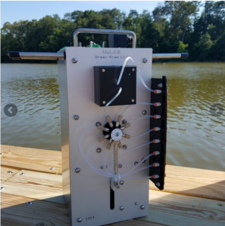
NuLab monitoring nutrients in a waterproof enclosure on a Florida bay
