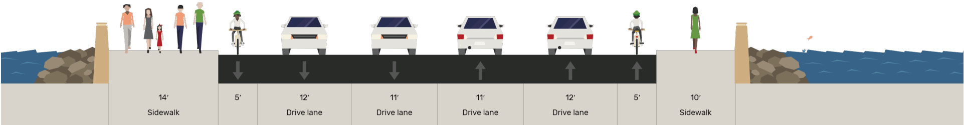
Existing Section (looking west)
