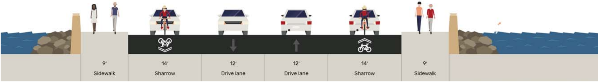
Recommended Section (looking west)
