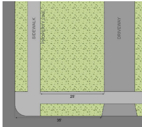
Figure 1: Access Distance From Intersections
