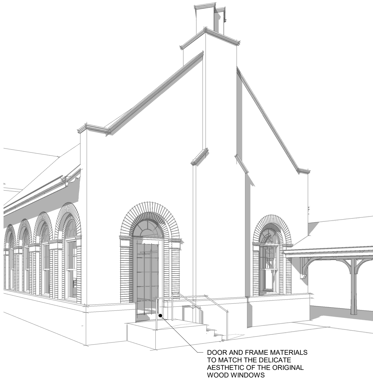
PROPOSED EXIT ONLY EGRESS DOOR AND STAIR
