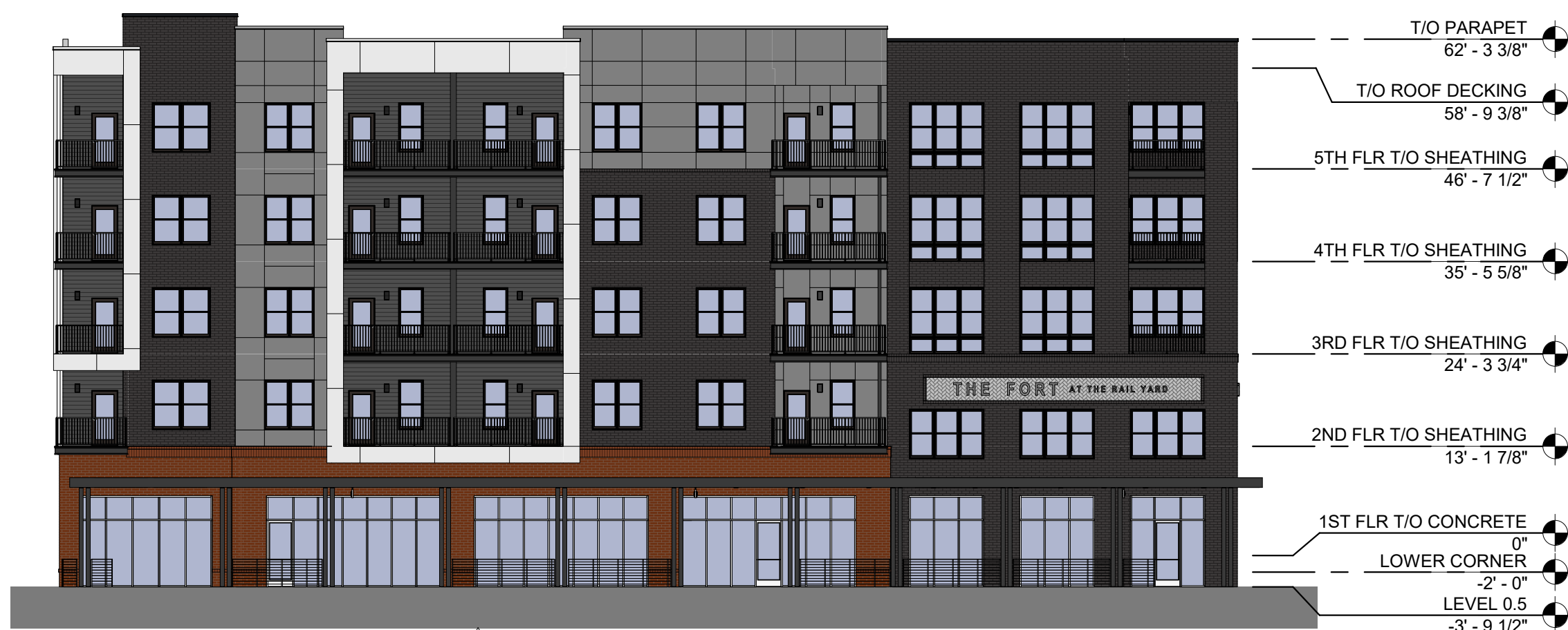
7 WEST ELEVATION - OVERALL - AREA A 1/16" = 1'-0"
