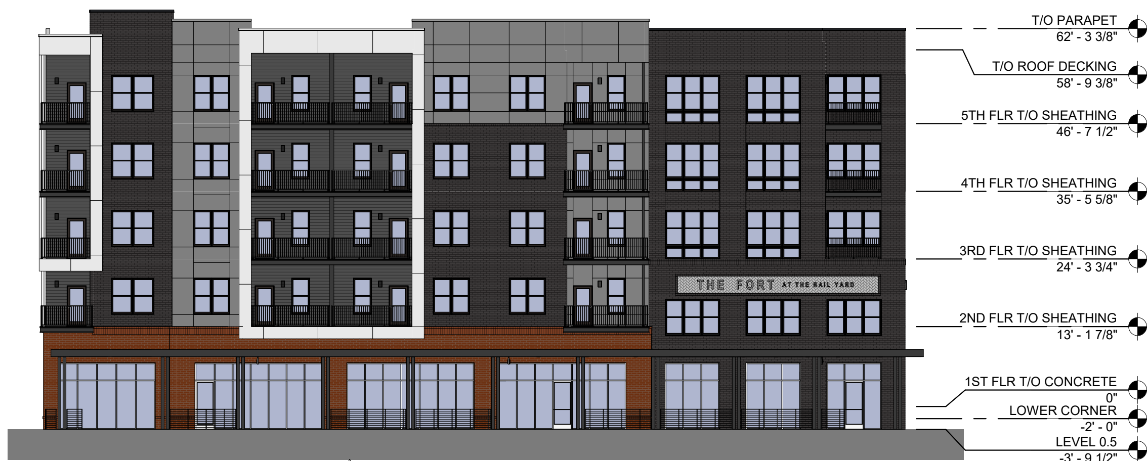
7 WEST ELEVATION - OVERALL - AREA A 1/16" = 1'-0"
