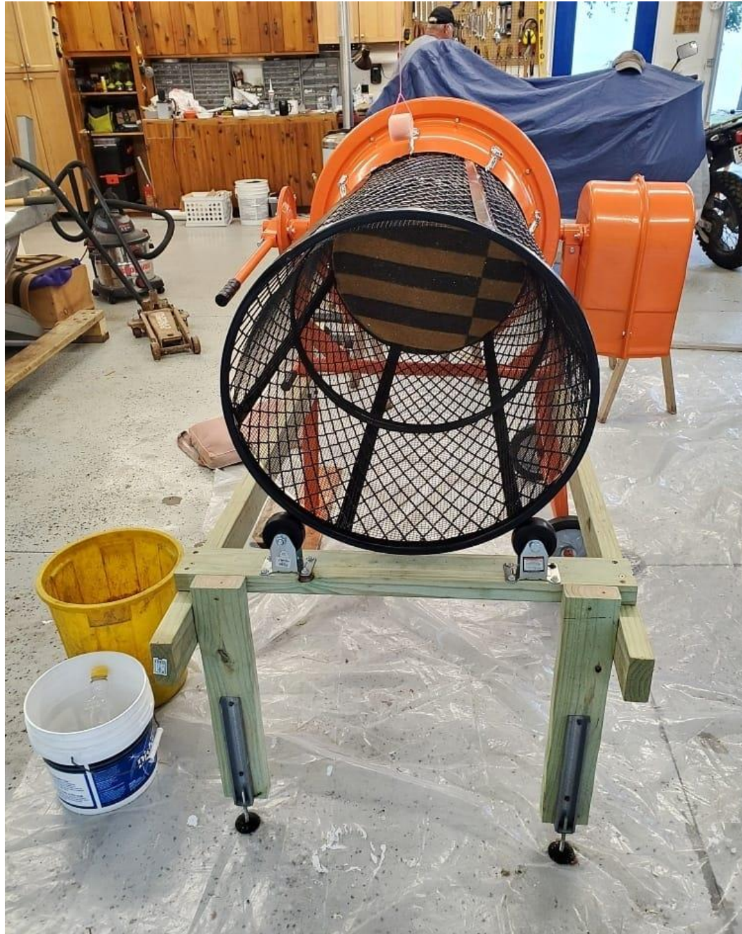
Our custom-built, automated compost sifter, which we use to sift our finished compost down to 1/4" in size.
