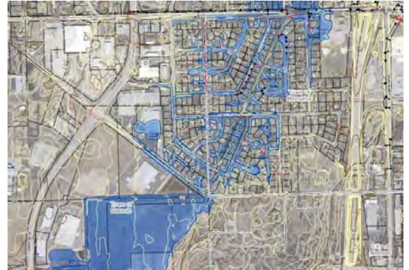
100-year flooding along Green Valley Waterway
