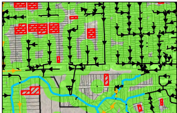
Identification of Areas without Drainage Infrastructure
