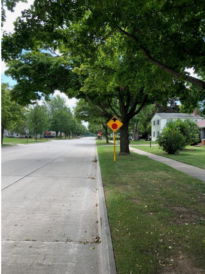
Example : Southbound Locust approaching Bond Street. Added Brite Side to post support panel on STOP AVANCE SIGN and Double up STOP SIGN at Bond Street
