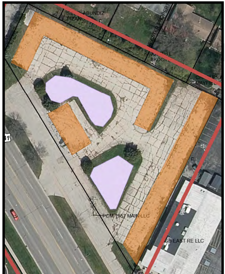
Figure 3: Proposed site with rain garden areas shown in purple and potential building footprints shaded in orange.
