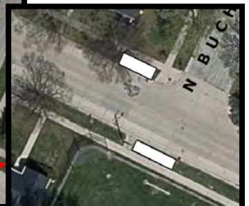
Figure 3: Proposed site showing bioswale areas as white rectangles.
