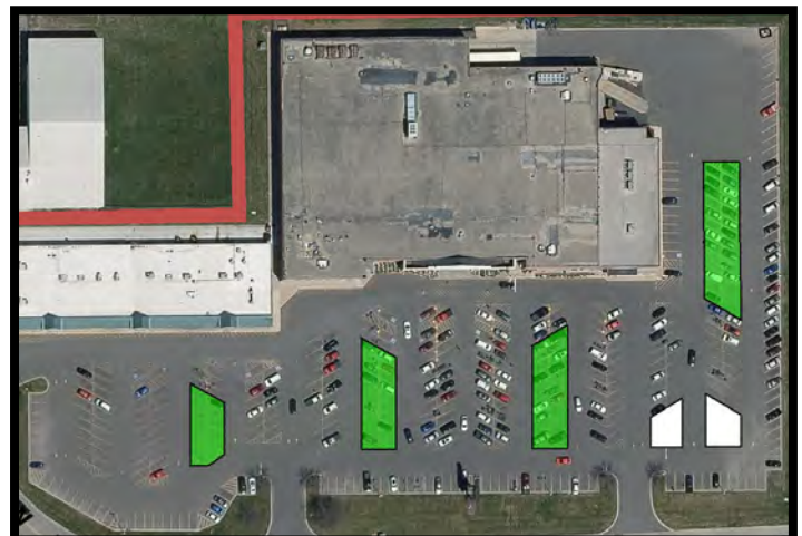
Figure 4: Proposed site with permeable paver areas shaded in green and bioswale areas in white.
