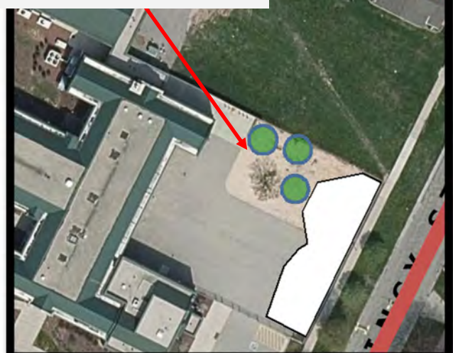
Figure 3: Proposed site with bioswale area shown in white and tree shown by green and blue outlined circles.
