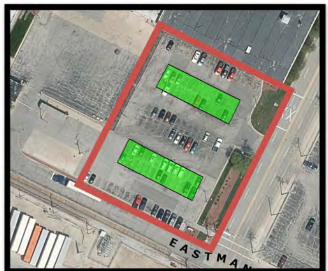
Figure 3: Proposed site with permeable pavement areas shown as green rectangles.
