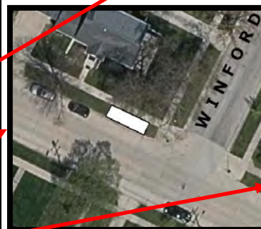
Figure 3: Proposed site showing bioswale areas as white rectangles.
