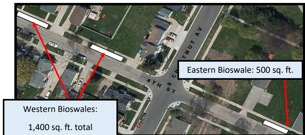
Figure 3: White rectangles indicate intended bioswale location
