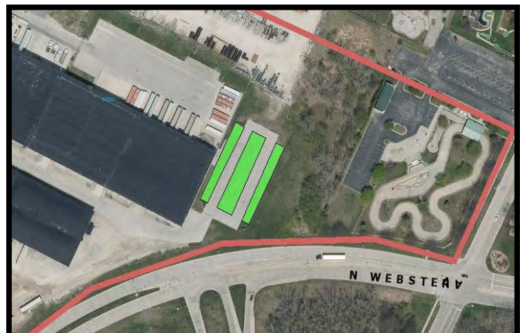
Figure 3: Northeast section of project site with proposed permeable pavement areas as green rectangles.
