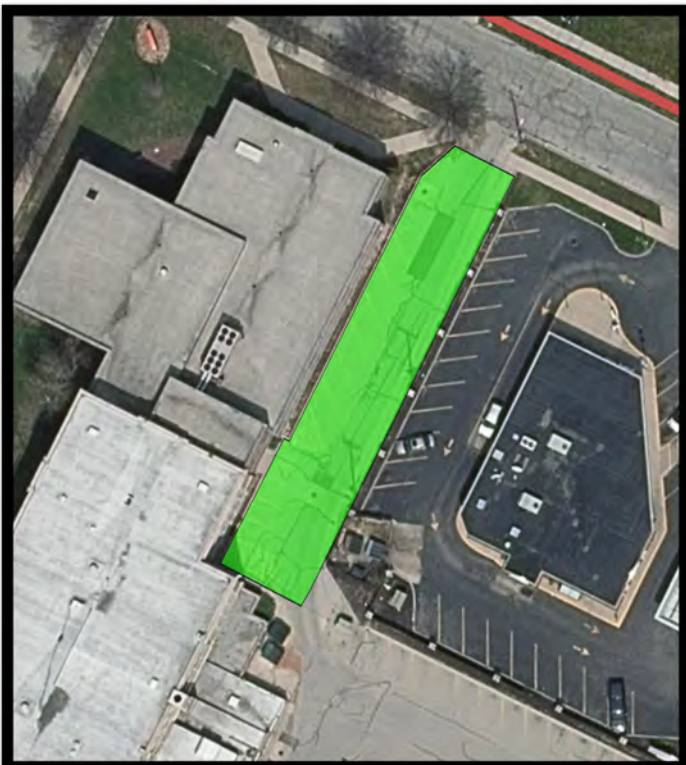
Figure 5: Proposed site with permeable paver area shown in green.
