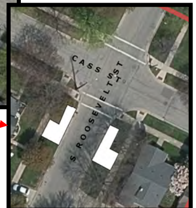
Figure 3: Proposed site showing bioswale areas as white rectangles.
