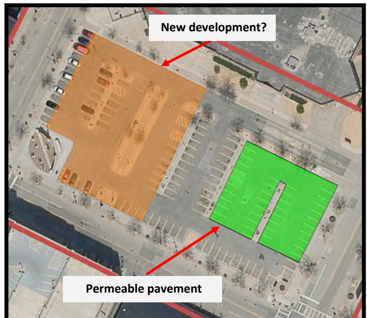
Figure 3: Proposed site with permeable pavement areas shown as green rectangles. Area that could be used for new development is shaded in orange.
