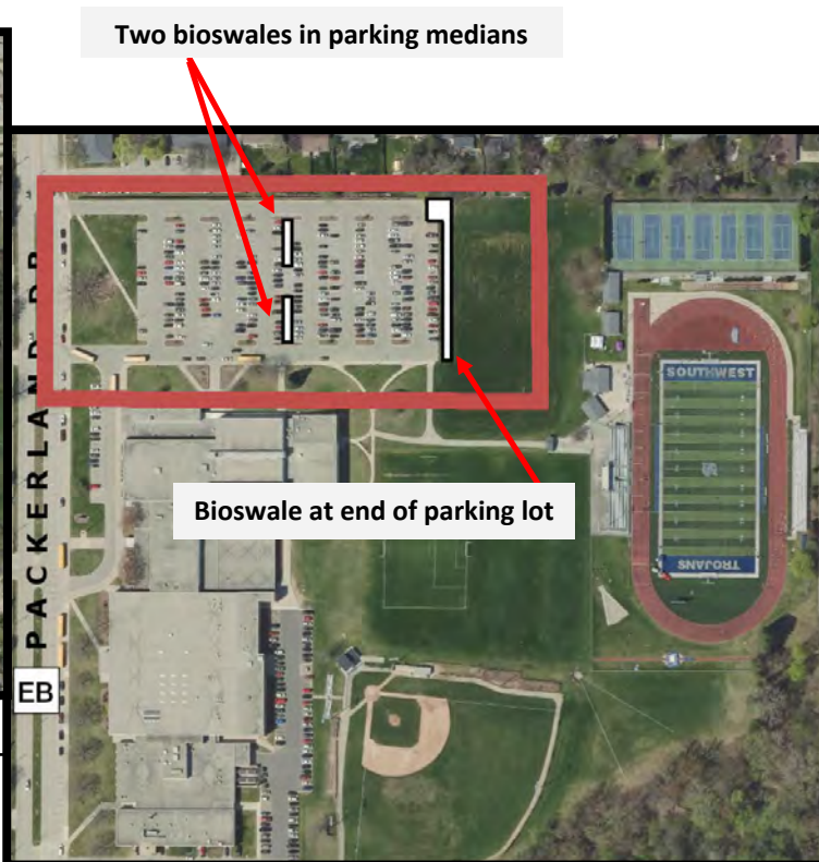
Figure 2: Proposed site with bioswales shown as by white rectangles.
