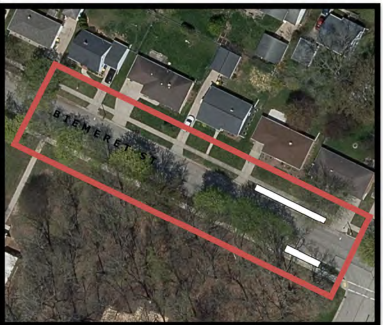
Figure 3: Proposed site. The bioswales are shown as white rectangles.
