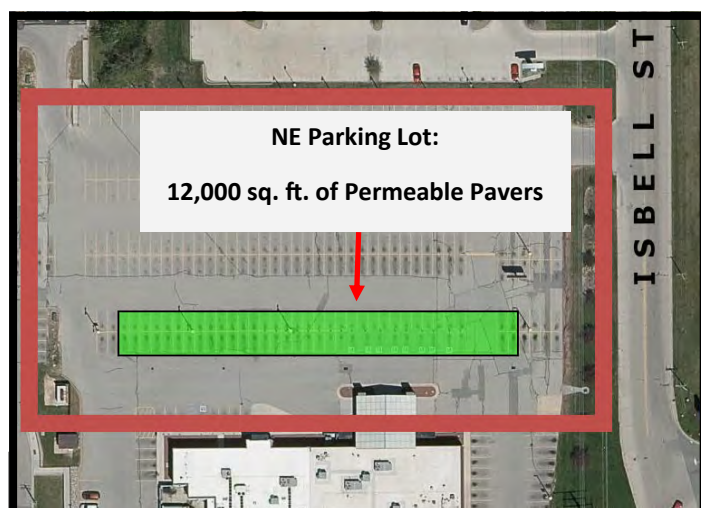
Figure 3: Proposed site with permeable pavement areas shown as a large green rectangle.
