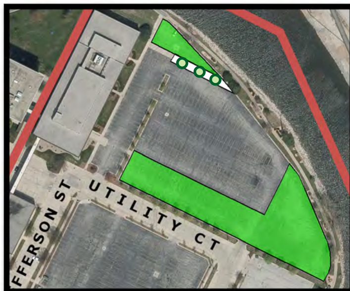
Figure 4: Proposed site with permeable paver areas outlined and shaded in green and bioswale areas in white with trees.
