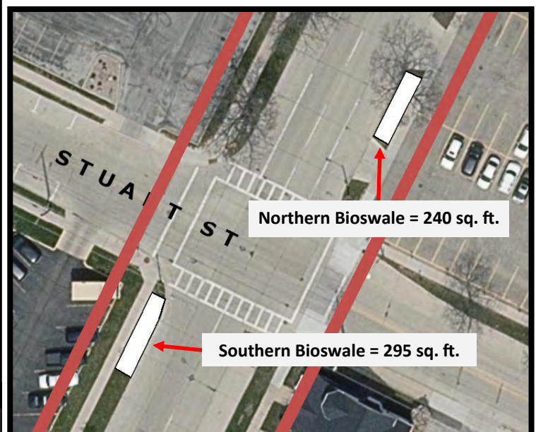
Figure 3: Proposed site with bioswales shown as white rectangles.
