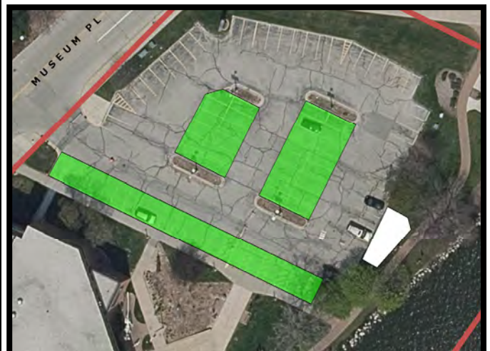
Figure 4: Project site with proposed porous pavement areas denoted by black rectangles.
