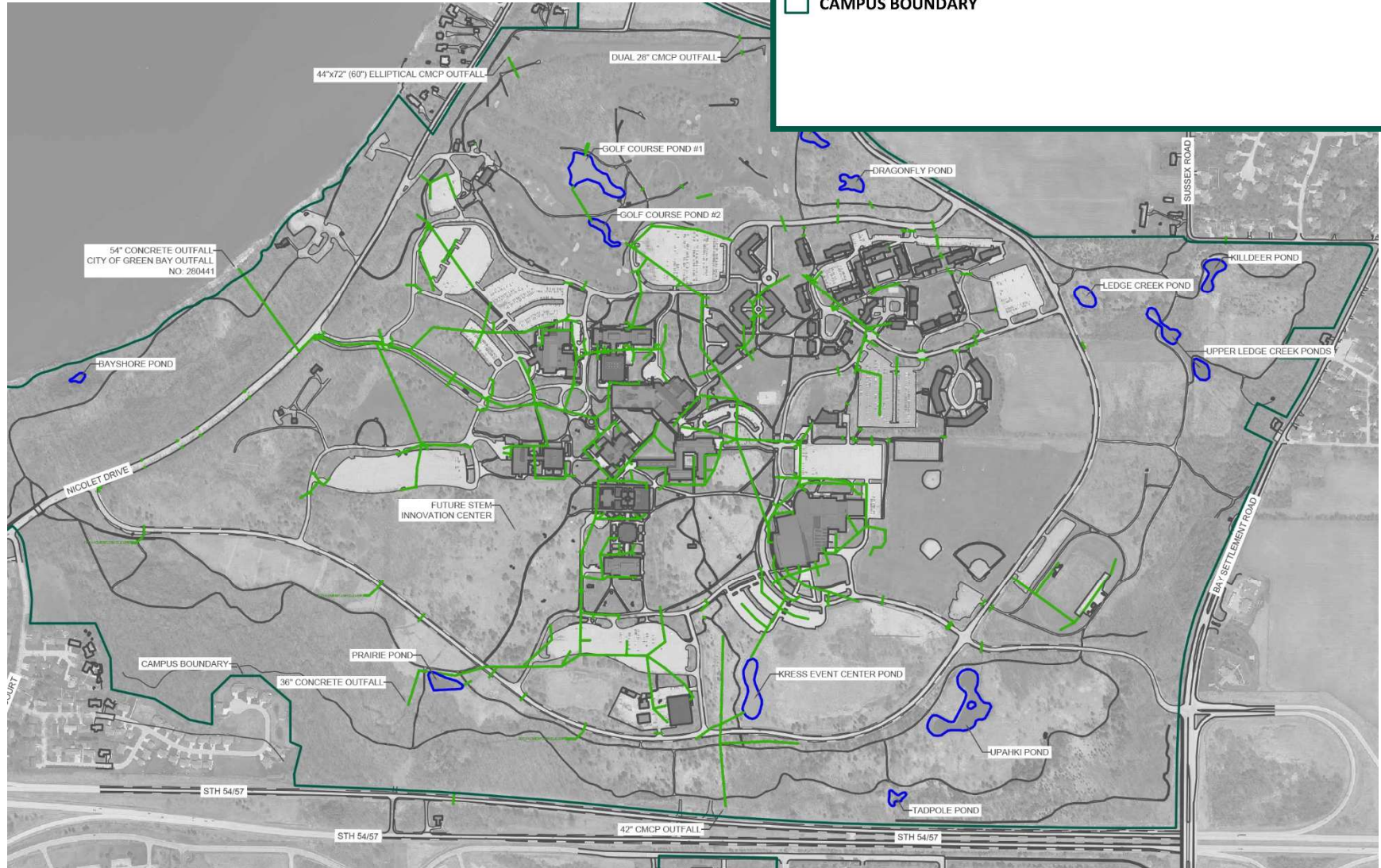
Figure 4.8-1: Existing Campus Stormwater Ponds
