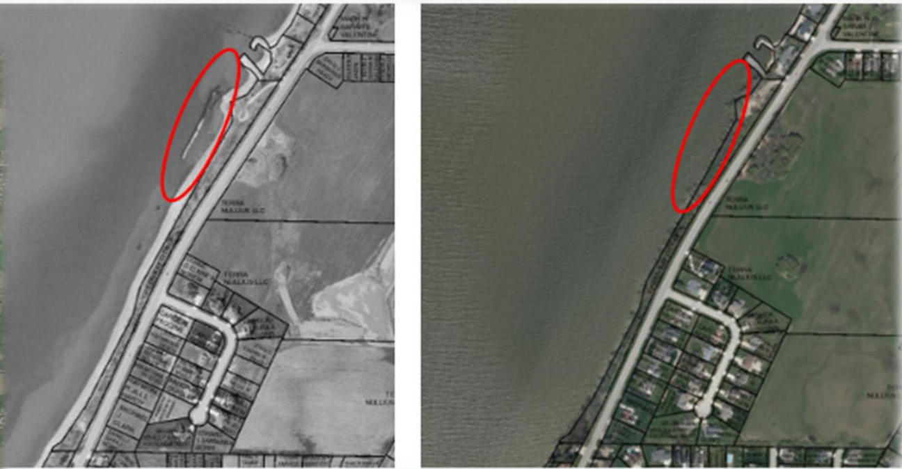
Left: walleye reef shortly after construction in April 2000 (176.14 m monthly average water level) Right: walleye reef in May 2020 (177.38 monthly average water level). The left and right image reflect a change of over 1.2 m/4 ft in water levels.
